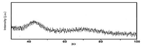
Fig. 2. The X-ray diffraction patterns obtained for amorphous alloy strip  $Co_{22}Y_{54}Al_{24}$
