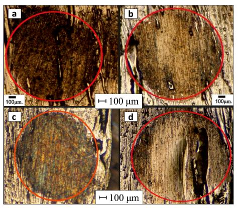
Fig. 3. Wipe the shiny surface of the tape after 1h (a), after 2h (b) and the matte side after 1h (c), after 2h (d)
